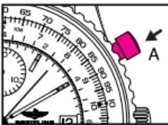
2. To interrupt the measurement, press pushpiece A once more. To restart the time measurement, press pushpiece A. This procedure makes it possible to add several short times.
