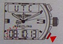
Press pushpiece B briefly: the H and MIN on the display flash in turn.
